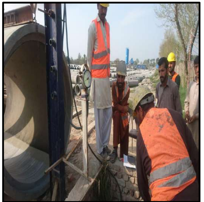
Picture 26: 3- Edge Bearing Test of RCC Pipe
