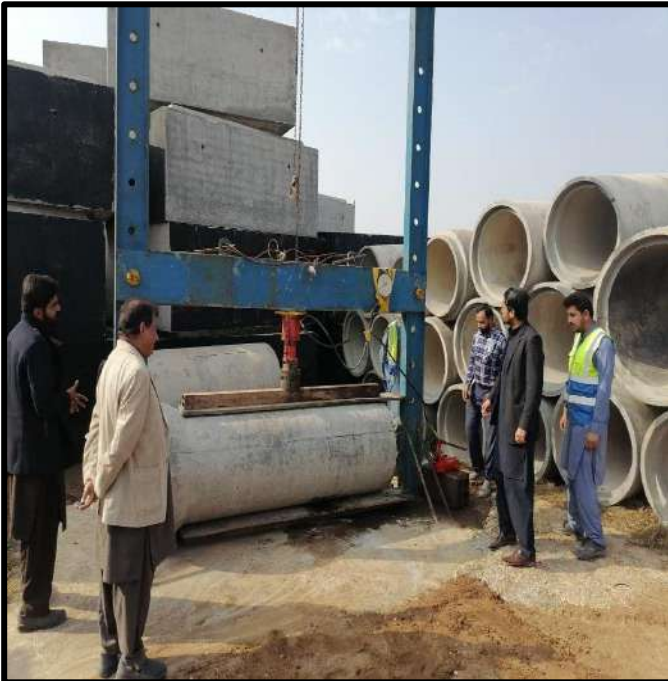
Picture 59: 3- Edge Bearing Testing for RCC Pipe
