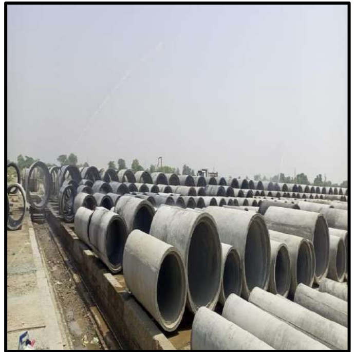
Picture 40: Curing of RCC Pipe at RCC Pipe Factory Lot-04
